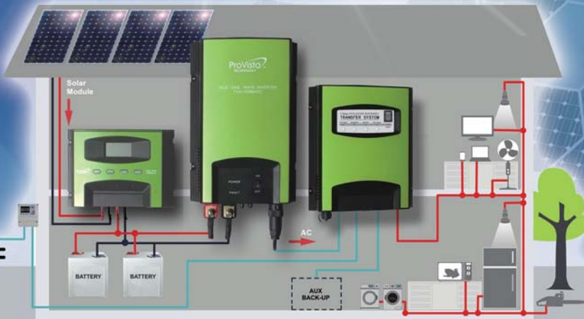
SOLAR CONTROLLER, INVERTER & TRANSFER BOX
